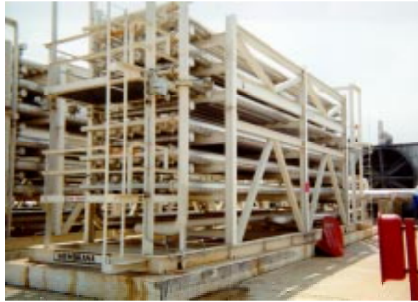
Figure 7: Skid-Mounted Membrane Tubes Containing Spiral-Wound Elements
